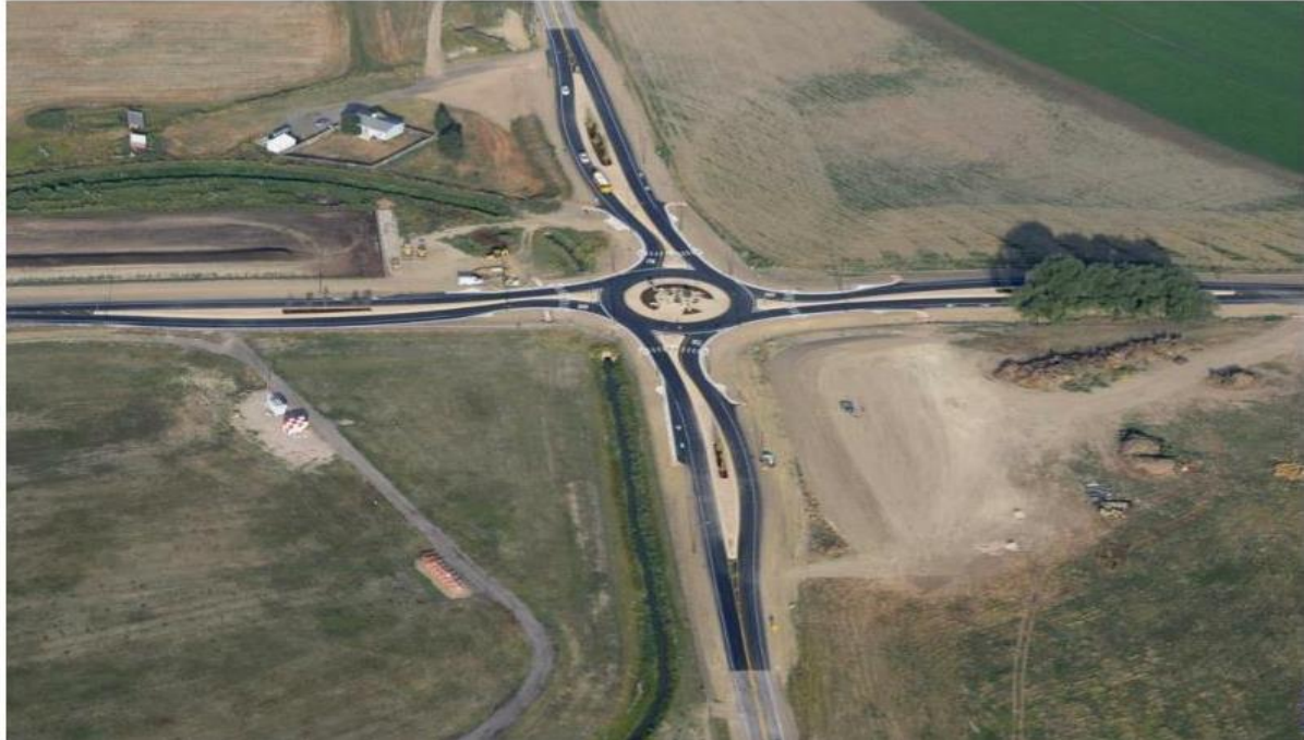
Figure 40 Rural Single-Lane Roundabout
