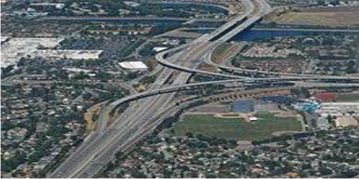
Figure 7 Three-Way Directional Interchange
